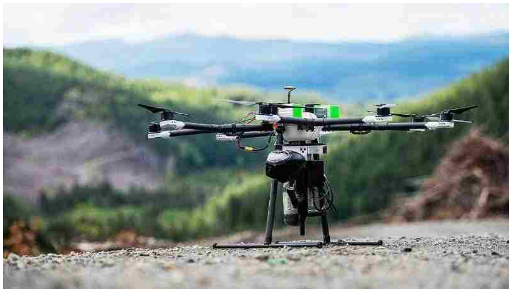
Figure 24. Biocarbon Engineering seed planting drone 63
