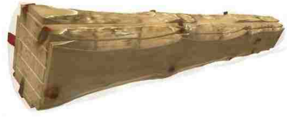
Figure 21. 3D model of log produced by CT scan for most efficient milling 58
