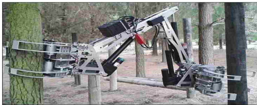
Figure 28. Tree-To-Tree Swinging Forest Harvester 68
