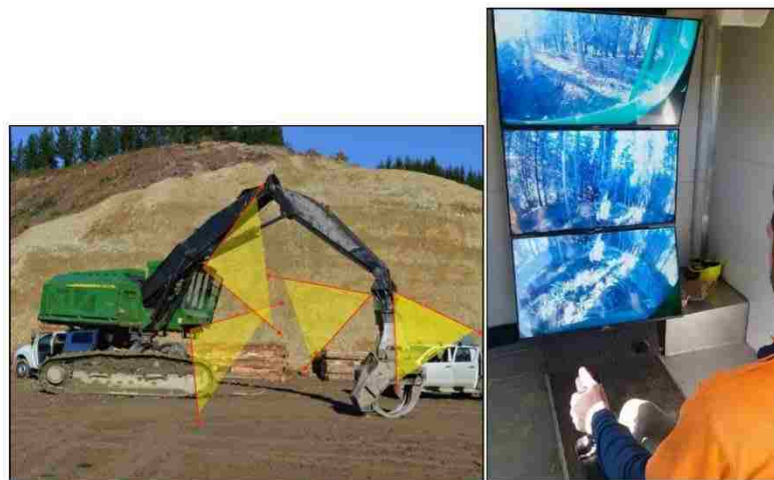
Figure 25. Camera Locations and Remote Control Apparatus 65
